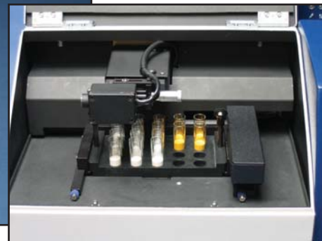
Reflectance Mode for Vials and Tablets
