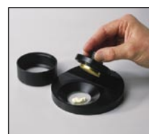
0.1 mm Gold reflector 0.2 mm Gold reflector 0.5 mm Gold reflector For use with either slurry cup or small sample cup.
